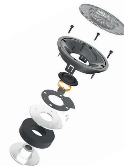
Construction of the tweeter driver of the Debut 2.0 Series.
